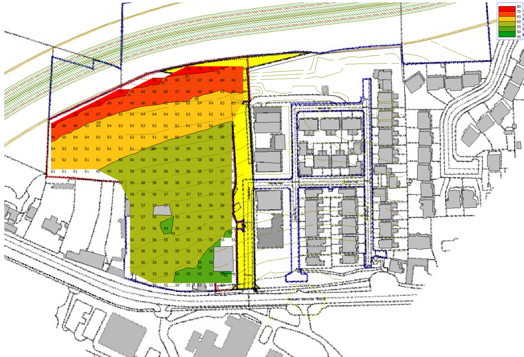
Figure 6 L_{Aeq,16hr} Daytime Road Traffic Noise Levels, dB(A) – 1.5m AGL without development
